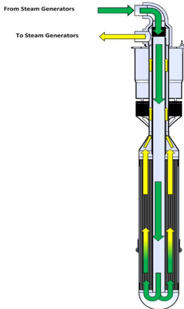
Each IHX is nominally 2m diameter at the shell, 2.7m maximum diameter and 17.5m overall height. Flow into and out of the heat exchanger is coaxial with differential thermal expansion managed by bellows at the top of the central cold leg. The IHXs are expected to be fabricated from SS304H Austenitic Steel.
