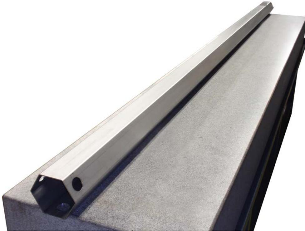
Strict dimensional and tolerance requirements for the tube hexagonal profile, wall thickness, and straightness will be imposed by the product drawing. The duct tube has an outer dimension of approximately 140 millimeters and a length of approximately 4 meters.
