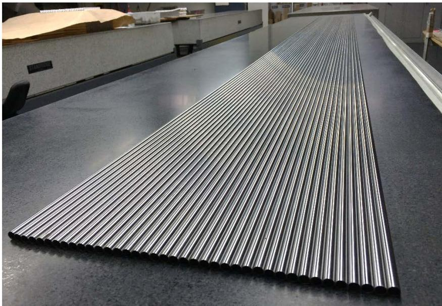
Strict dimensional and tolerance requirements for the tube diameter, wall thickness, and straightness will be imposed by the product drawing. Multiple cladding tube sizes are needed for the various core components. The principal quantity of tubes has an outer diameter of approximately 8 millimeters and a length of approximately 3.5 meters. The other cladding tube
