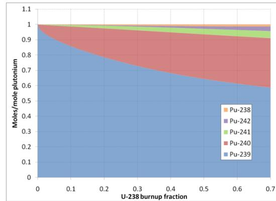
Fig. 8. Fast reactor plutonium vector evolution.
