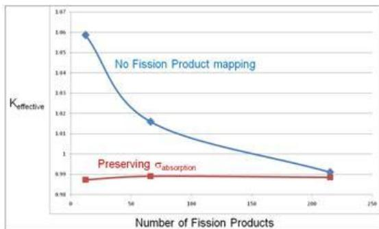
Fig. 3. Criticality of a simplified high burnup system as a function of the number of fission products kept in the Monte-Carlo transport simulation. Mapping the Cinder90 fission products onto those kept in a way that preserves their macroscopic absorption cross-section allows most scoping calculations to run with keeping only 12 fission products in the transport calculation.
