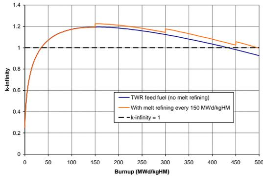
Fig. 6.  $k$ -infinity evolution for a representative TWR fuel-load.
