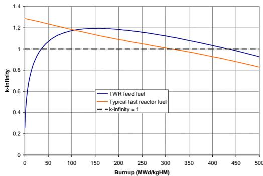
Fig. 7.  $k$ -infinity evolution for TWR and typical fast reactor fuels.
