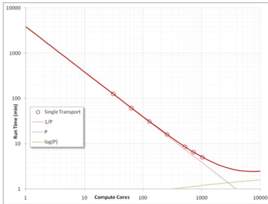
Fig. 4. The run time of a high-precision neutron transport problem as it depends on the number of compute cores applied. The red line through the points shows an estimate of how the curve might continue beyond 1,024 cores.
