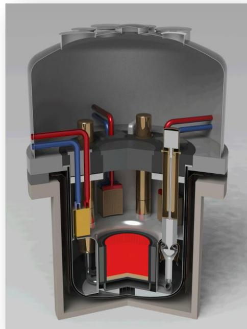
Fig. 1. Possible practical engineering embodiment of a TWR.
