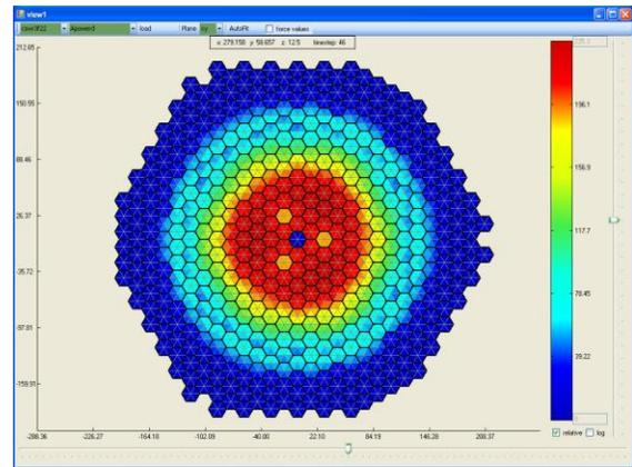
Fig. 5. XTVIEW - TerraPower's 3D visualization tool. Slider controls allow the user to scan through the reactor, in space and time, to understand its performance.
